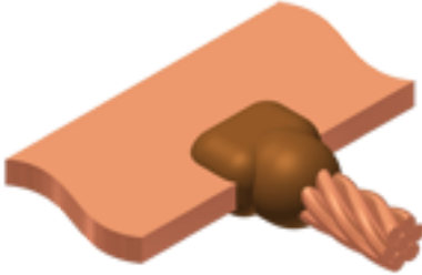
Horizontal Cable Horizontal Bus Bar
